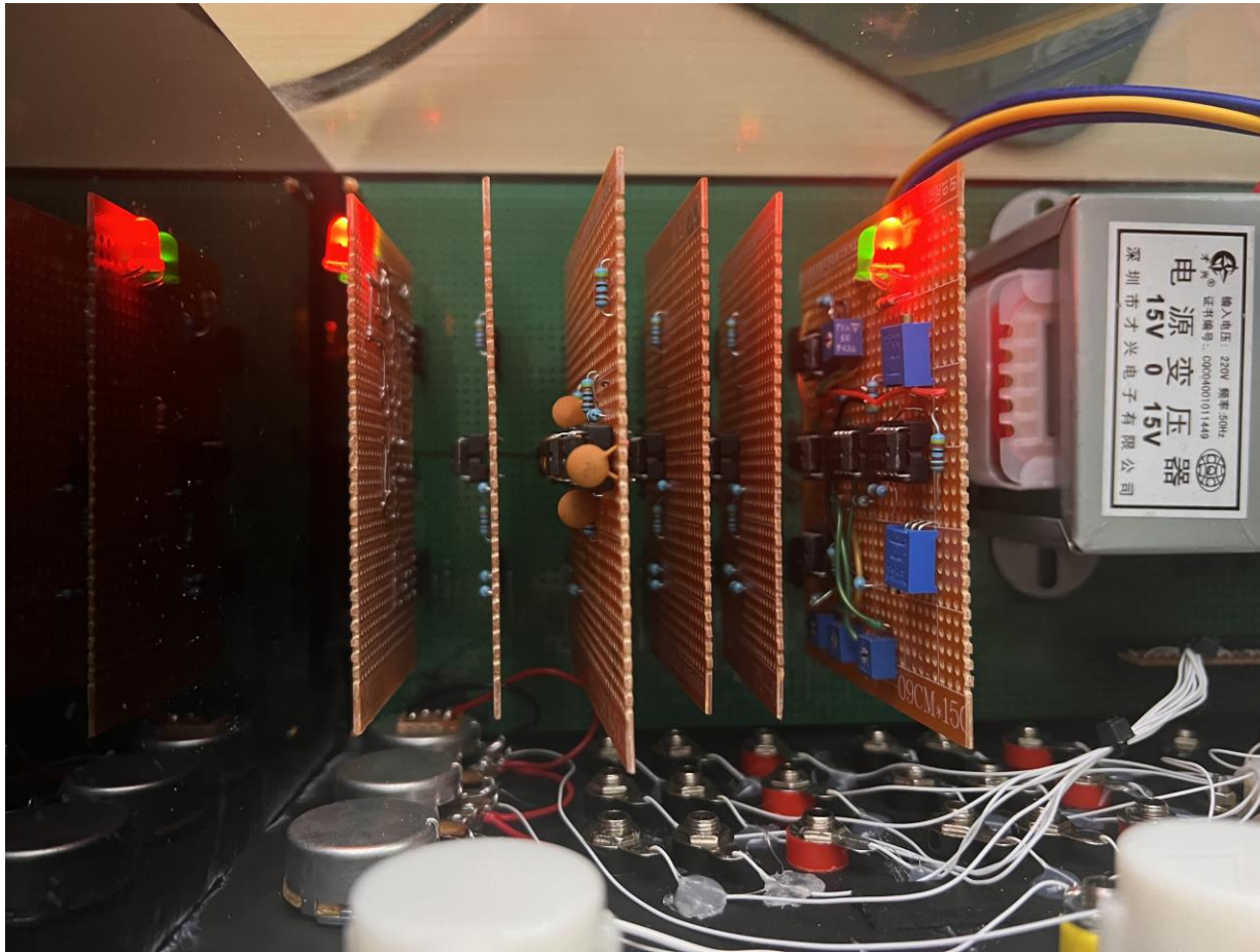
Figure 82. LED added on each end of the modules
