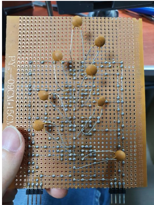
Figure 79. Connecting decoupling Capacitors to +12V/-12V inputs of the module
