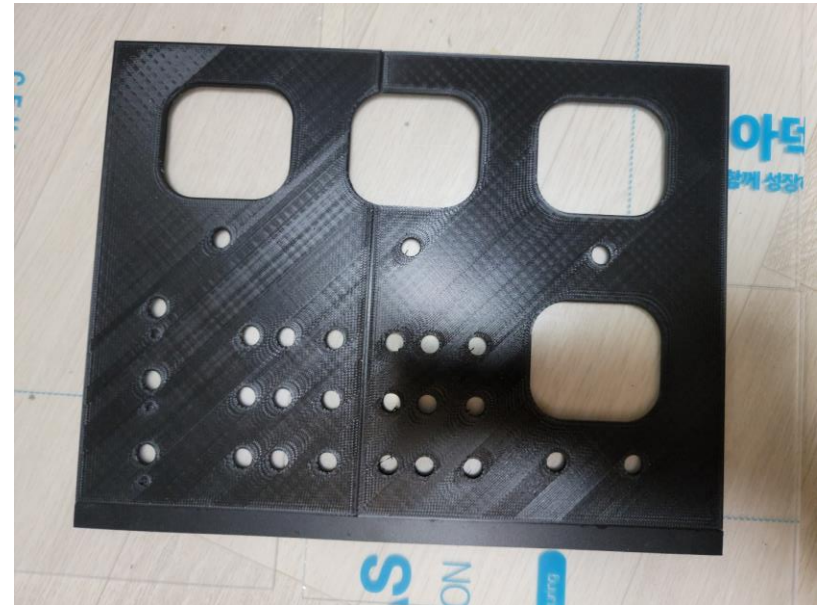
Figure 57. Front Panel designed on Fusion 360 (Left) and Printed Front Panel Using 3D Printer (Right), Source: [12]
