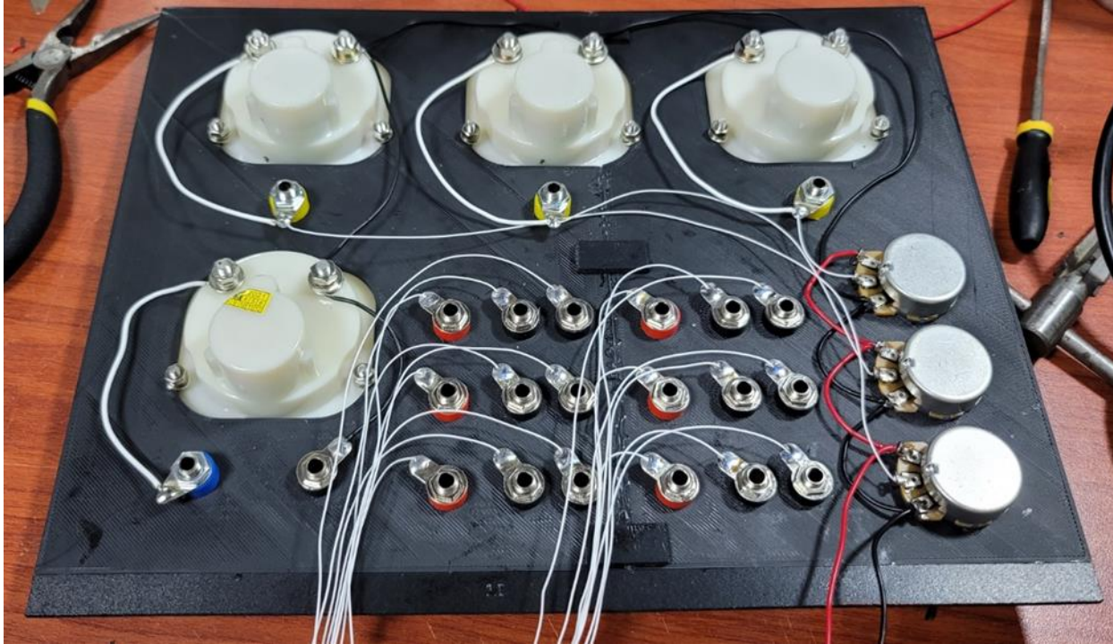
Figure 58. Soldering the Panel of the Calculator
