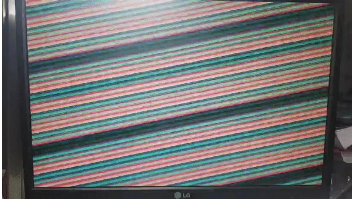
Miscalculated Timing on H_sync & V_sync Pulses
