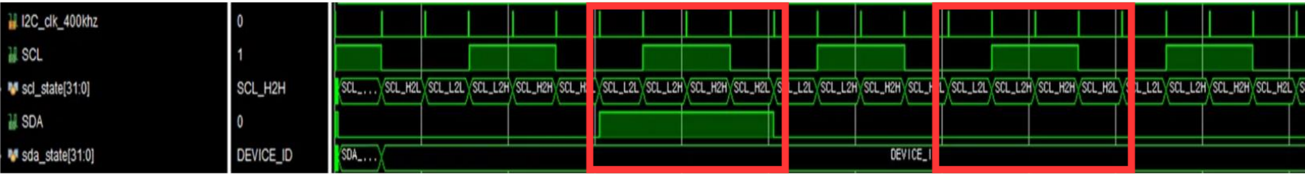
▲ SCCB Protocol Bit Level Timing (1's and 0's)
